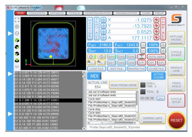
After completing the work process, the system automatically moves to the workpiece zero point (X, Y) and to the top Z-axis position. **Turn off the 3D print head** and move the gantry to the rear end of the desktop system.
