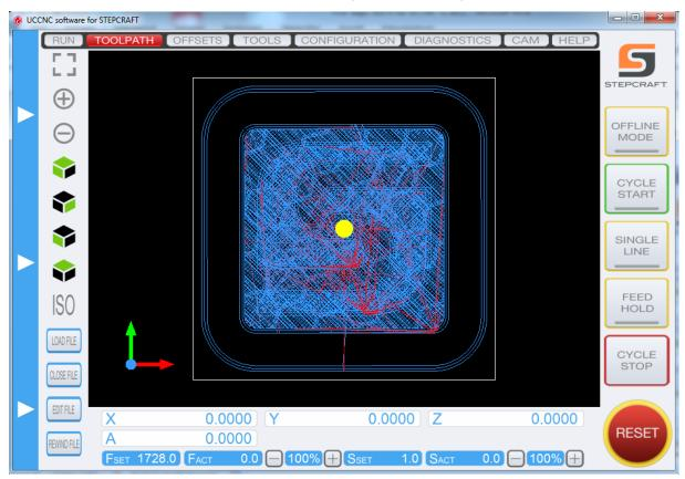
The file consists of a 3D pattern of the STEPCRAFT logo. The workpiece has a size of 30 x 30 mm (approx. 1.25 inch x 1.25 inch).
