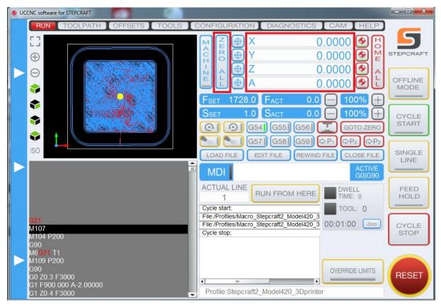
The workpiece coordinates are then X = 0.000, Y = 0.000 and Z = 0.000. The yellow dot in the toolpath preview marks the actual position of the machine and is located in the centre of the workpiece as expected.
