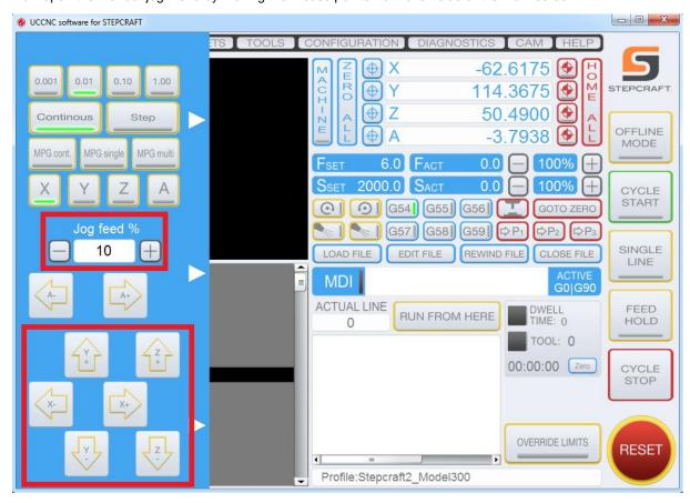
Move the cursor to the arrow keys and place the machine carefully in the middle of the workspace of the system. To increase the moving speed you can adjust the jog feed.
