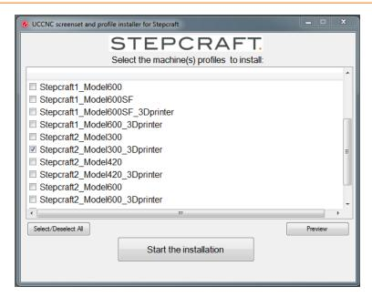
Start the installation. The installation will create a desktop icon and prepares, for example, different technical parameters for the 4<sup>th</sup> axis. In the 3D print configuration a plugin will be installed additionally to control the 3D print head.
