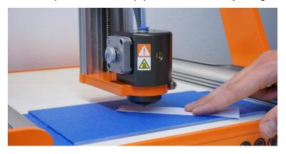
Once the nozzle touches the paper, save that point again as the workpiece zero point X/Y/Z by pressing "Zero all".
