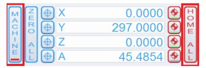
The machine will start driving all axes now, beginning with the Z-axis, until it reaches the reference switch of each axis. When the homing is completed, the machine (seen from the front) features (X) on the left, (Y) at the rear and (Z) at the top.
