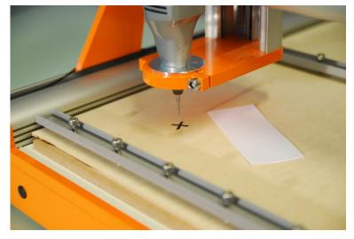
Move the paper back and forth with your fingers. Once the cutter touches the paper, save that point again as the workpiece zero point X/Y/Z by pressing "Zero all":
