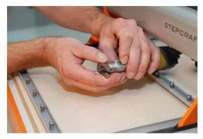
After the insertion tool has been fixed in the collet, the spindle has to be clamped into the machine. The machine has a 43 mm tensioning system. You need a tool adapter if the tool neck is smaller than 43 mm. Lock the spindle, or the spindle with tool adapter, into the tensioning system with an Allen key.
