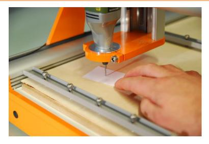
After this move the Z-axis manually up to approx. 20 mm above the workpiece.
