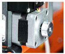
Important: Make sure that the stroke motor is not activated during creasing. The respective settings have to be adjusted depending on the control / CAM software used. Please test your program first with sufficient distance to the workpiece. An oscillating creasing wheel can lead to damage to the machine and to your OTK-3.
