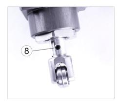
The creasing wheel should be operated in the upper dead center. For this purpose, set the creasing wheel to the highest position by manually turning the hand wheel of the stroke motor.
