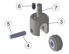
Insert the mounted unit into the OTK-3. The Weldon clamping surface (7) has to point towards the clamping screw (8). Hold the creasing wheel in this position and secure the unit with the clamping screw.
