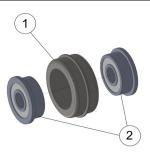
Place the creasing wheel with the ball bearings inside the body (3). Guide the shaft (4) through the body and the creasing wheel. Take care that the shaft's recess is located on the side of the threaded pin (6). Fasten the shaft with the threaded pin.
