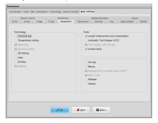
**Step 2** – Close WinPC-NC and restart the program. The new tab *Sensor* will now appear under *Parameters* > *Basic Settings*. Select the new tab and enter the sensor value.
