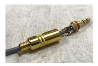
The Tool Length Sensor can now easily be plugged into the jack socket of the STEPCRAFT mainboard.
