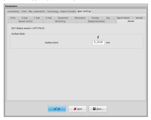
**Step 3 –** Visit *Parameters > Basic Settings > Signal Wizard > Inputs* and define *I221 Surface sensor* as *LPT1 Pin 10*.
