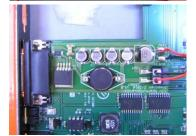
9. Connect the constant voltage regulator to the port of the 4th Axis Module. Make sure to insert the connection cable of the regulator exactly as pictured!
