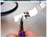
Take the cable channels and attach them to the gantry upright. When upgrading an existing machine, cut a small slot into the upper cable channel prior to attaching it.
