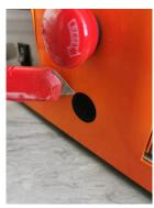
2. Pull the wire of the switch through the hole and tighten the switch from inner side of the front panel.
