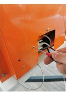
8. Strip the cable ends and connect them according to enclosed connection plan to the enclosure mainboard. Then remount the board into rear panel of the enclosure.
