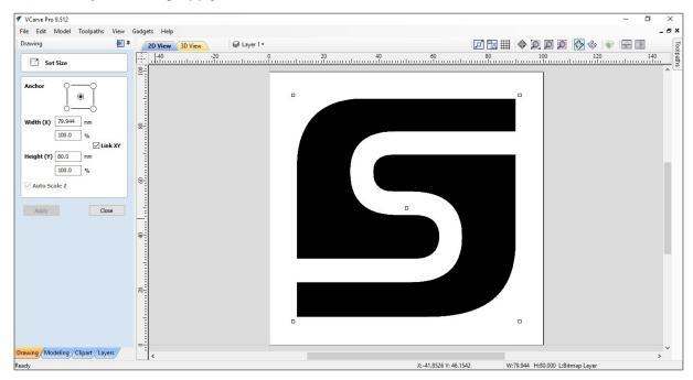
In the next step vectorize the logo resp. the contour, meaning the transformation in clearly defined curves and lines. For this purpose, select the logo again by clicking the left mouse button. Select the tool **Create Vectors / Trace Bitmap** on the left side of the screen.
