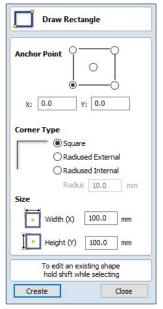
To draw the outer contour of the square, open the tool **Create Vectors** *I* **Draw Retangle**. As the anchor point is at the buttom left (workpiece zero point), the value for X and Y has to be 0. The width (X) and height (Y) are identical with each 100 mm.
