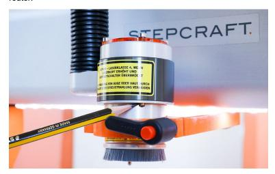
Be aware of the mounting position safety switch. Only when head is mounted correctly the safety switch is pressed down.
