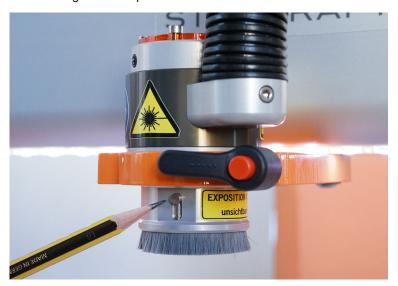
13. Jog to zero position Z of the work piece and check the Z height. Do corrections If the brushes do not touch the workpiece surface slightly (see section 4.1 or 4.2 regarding the parameters surface block (WinPC-NC) or double newZ (UCCNC). Repeat step 11 and 13 after manual movement of the Z-axis to a higher position and saving of the new parameter value.
