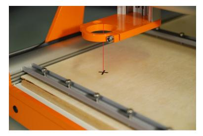
Save this using "Save to" as the zero point X / Y / Z.
