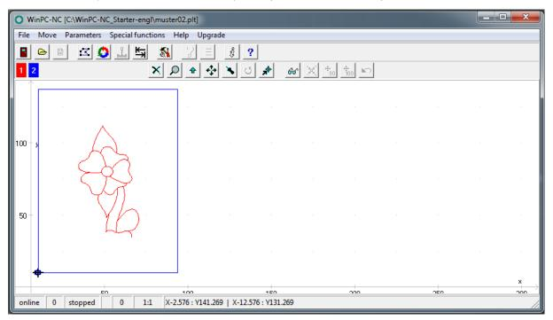
The file consists of an engraved pattern (red line) and the cut out of the workpiece (blue line).
