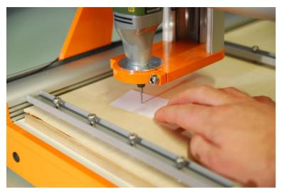
Move the paper back and forth with your fingers. Once the cutter touches the paper, save that point again as the workpiece zero point X / Y / Z:
