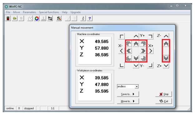
Double arrows = manual drive fast (X / Y axis at 30 mm / s, Z axis at 25 mm / s)
