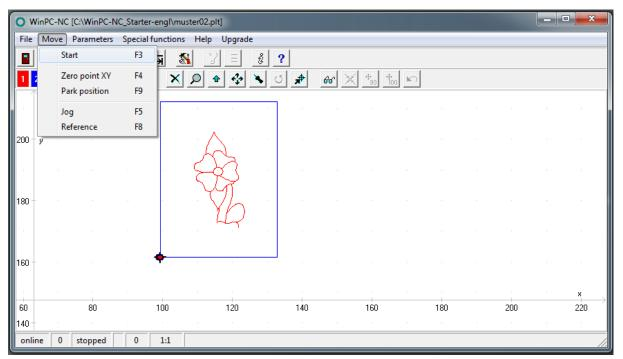
The machine moves to the workpiece zero point X = 0.000 and Y = 0.000, and then in the Z-axis for the first step (= engraving, red line) down to Z = 1.000. The work in progress is displayed in%:
