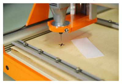
Take a piece of paper, put this on the work sheet and proceed slowly manually in the Z-axis downwards towards the workpiece:
