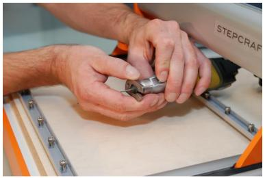
After the mill has been clamped in the spindle, set the clamping adapter (if required) in the 43 mm spindle taper of the STEPCRAFT. The milling spindle is used in turn in the clamping adapter. Lock the spindle in the spindle with the correct Allen key.
