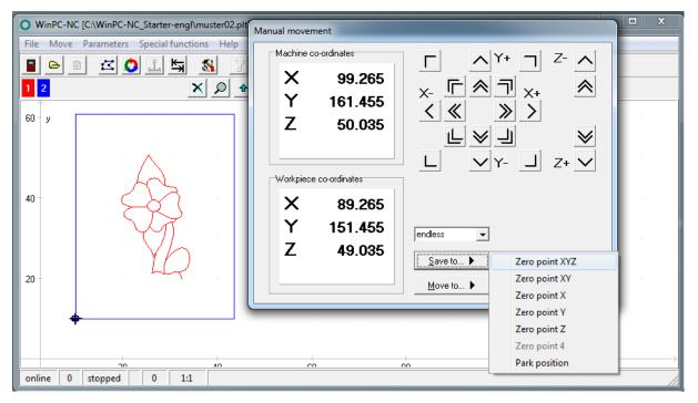
After saving the machine runs automatically 10 mm higher in the Z-axis (tool lift). The workpiece coordinates are then X = 0.000, Y = 0.000 and Z = -10.000.
