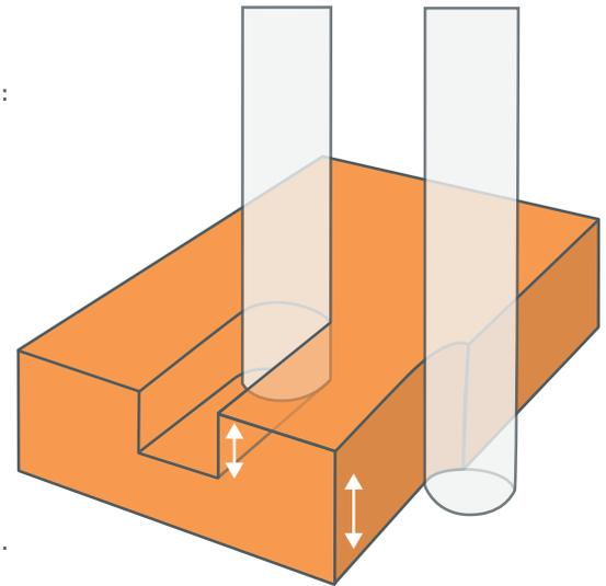
During contour milling we recommend a lateral infeed of approx. 25 % of the end mill diameter while applying 100 % immersion depth.
