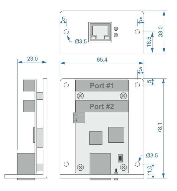
3.2 .Horizontal installation on the bottom of the mounting plate.
