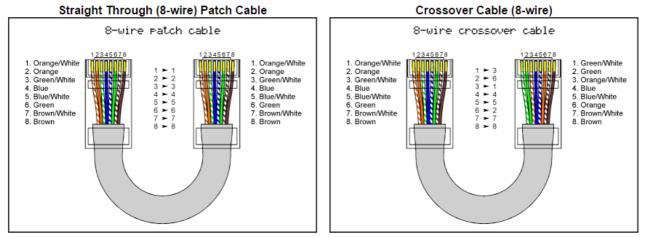
Use this cable for connection via router(s).
