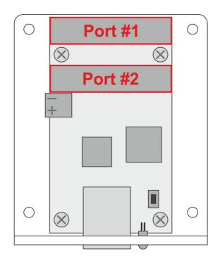
Both ports have 12 digital outputs and 5 digital inputs which is 24 digital outputs and 10 digital inputs in total.
