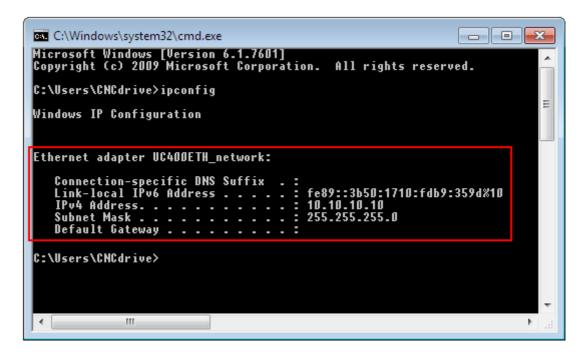
The UC400ETH network settings should be setup to fit the network settings on the PC side. To do the setup run the UCxxx\_utility.exe application which file can be found in the UCCNC software installation folder.
