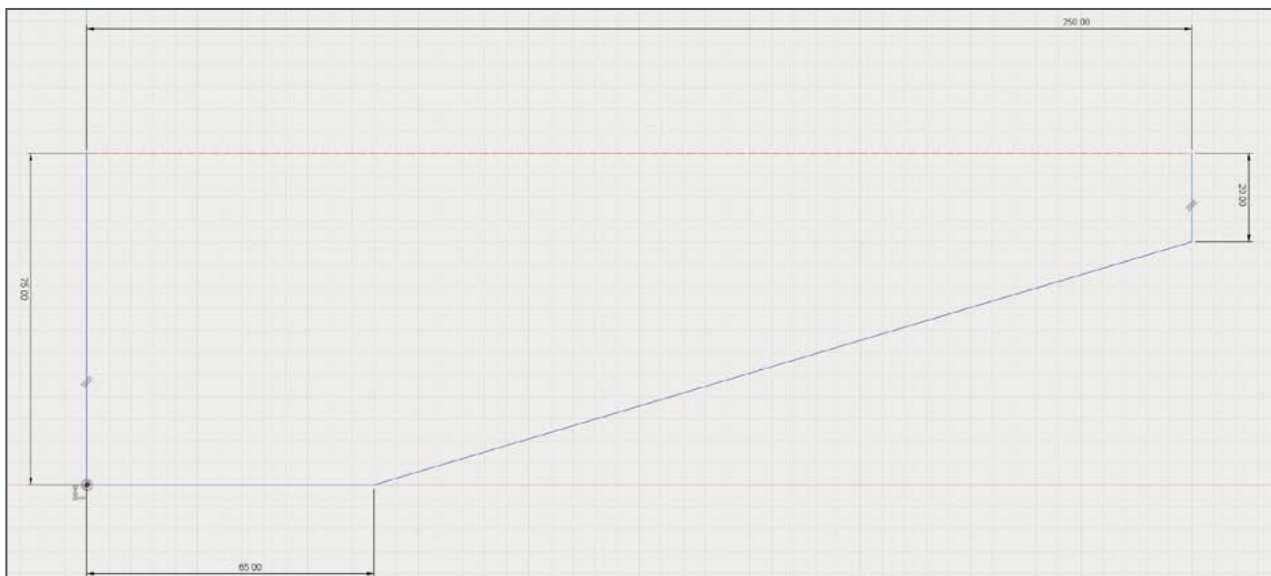
Fig. 82: Sketching the outer borders of the base plate
