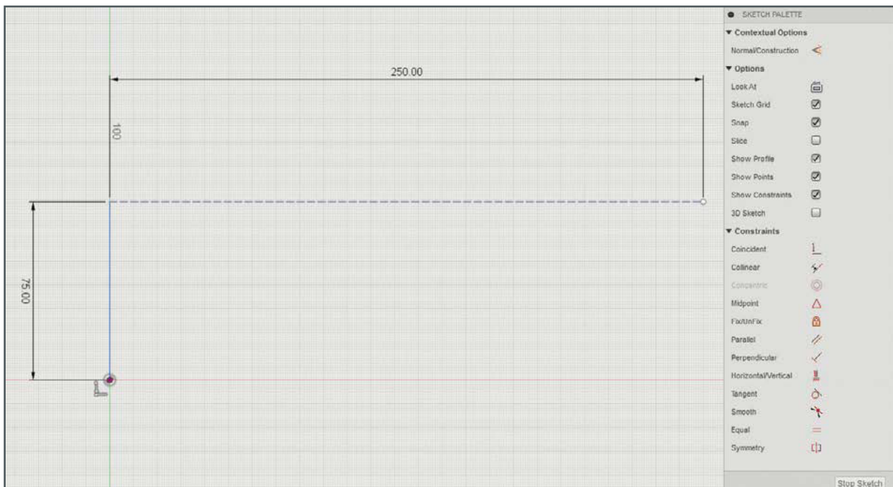
Fig. 81: Defining the axis of symmetry
